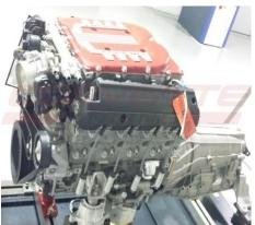
Zr-1 news has the engine at left as definitely an LT1-style, Gen V Chevy small block, as evidenced by the injector cover shape and the fact that the throttle body is consistent with those used on the C7's LT1.
